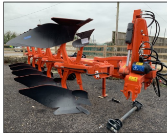
New Kuhn MM153, 5-Furrow plough, vari-width 16", 18", 20", auto-reset, full set of skimmers, rear discs, depth wheel. POA
